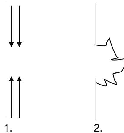
Figure 3. Spalling due to thermal stresses
