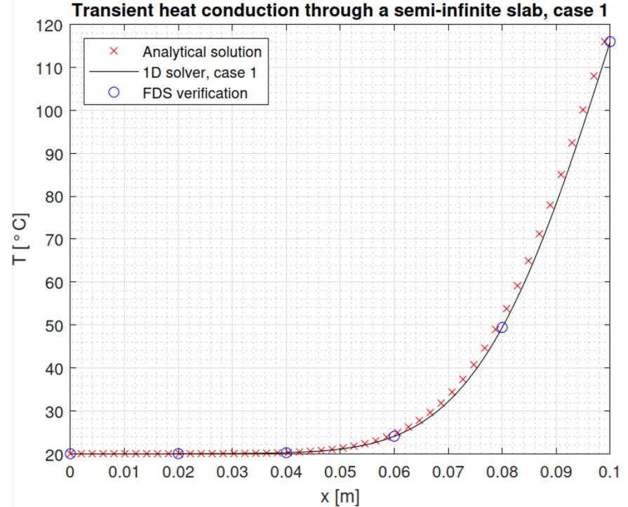
Figure 5. Transient heat conduction through a semi-infinite slab, analytical vs. numerical solution
