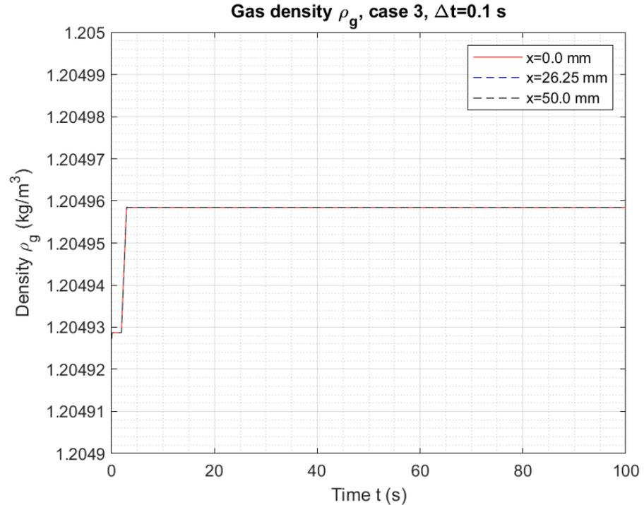
Figure 6. Gas phase mass conservation, sealed system
