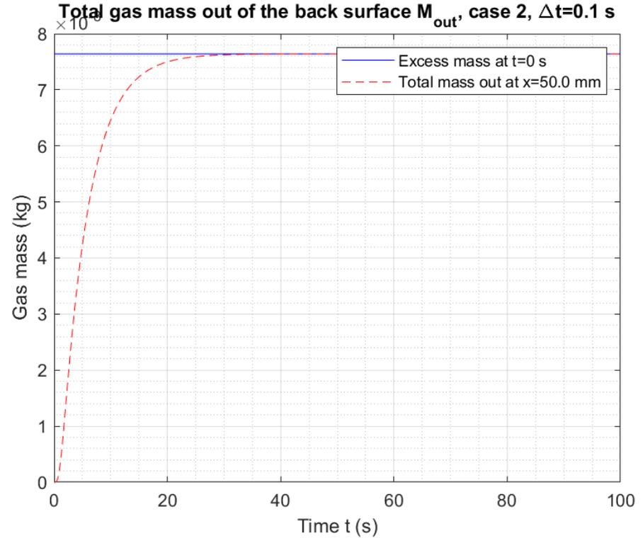
Figure 7. Gas phase mass conservation, mass flux through back surface
