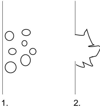
Figure 2. Spalling due to pore pressure
