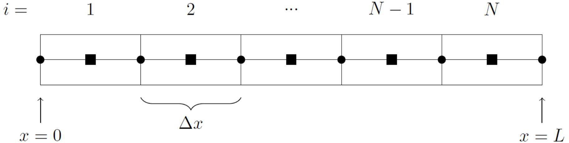
Figure 4. Discretization of the domain
